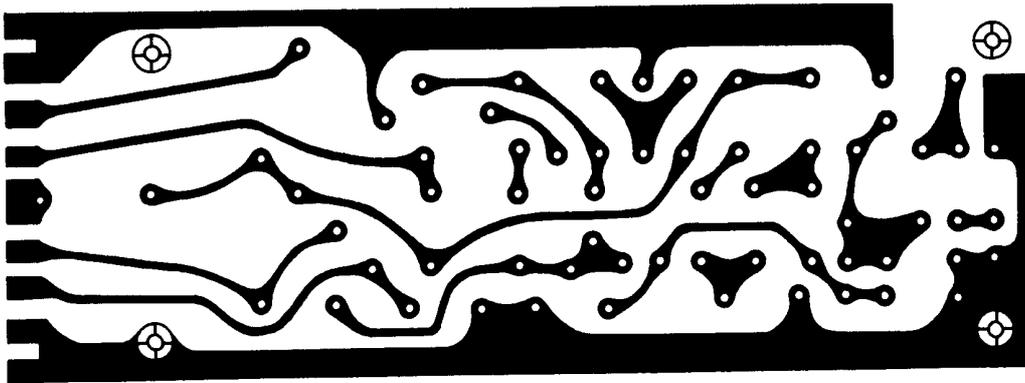
PLACA DE CIRCUITO IMPRESSO DO MÓDULO 20 a 40 WATTS - FIG.9 PÁG. 7
